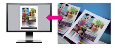
For soft proofing, a display with monitor calibration is recommended
