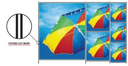
Regardless of any slight misalignment, when paper is introduced into the Digitrim, the cutter will automatically re-align itself to the image side!
