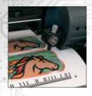
The automated contour alignment system OPOS stands for **O**ptical **Pos**itioning System. The OPOS X sensor technology senses marks on a wide range of materials.
