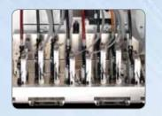
8 Latest Print Heads with Staggered Layout Advanced 508 nozzles print heads with staggered layout provides up to 100m<sup>2</sup>/h by 4 colors / 3 pass mode.
