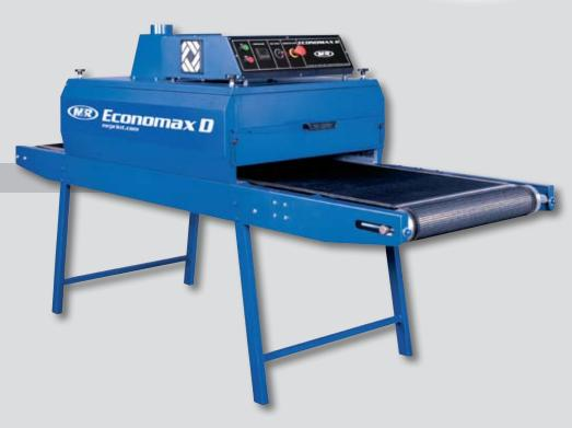
Easy to own and economical to operate, Economax D is the ultimate affordable, space-saving textile dryer. It's equipped with a 61 cm (24") belt. Not only does it have the highest production capacity in its class, it's also the most energy efficient. Heavy-duty thermal insulation prevents heat from migrating into the workplace, while CoolSkin™ technology leaves the dryer skin cool to the touch. Fast cure rates and high product throughput maximize dryer capacity and minimize per-unit cost.
